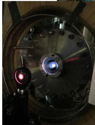
Plasma mirror device for FRC (Field Reversal Configuration) – RF heating for quasi-steady state magnetized cylindrical plasmas *Sam Cohen group @PPPL*
