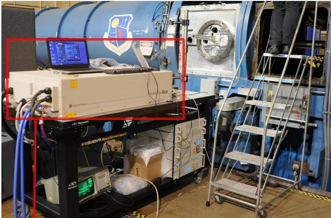
The laser system, optics and opto-mechanics components are installed on a transportable table placed in close proximity to the tunnel.
